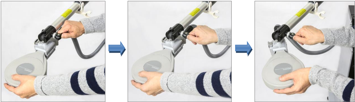
Figure 10. Changing the angle of the transducer
