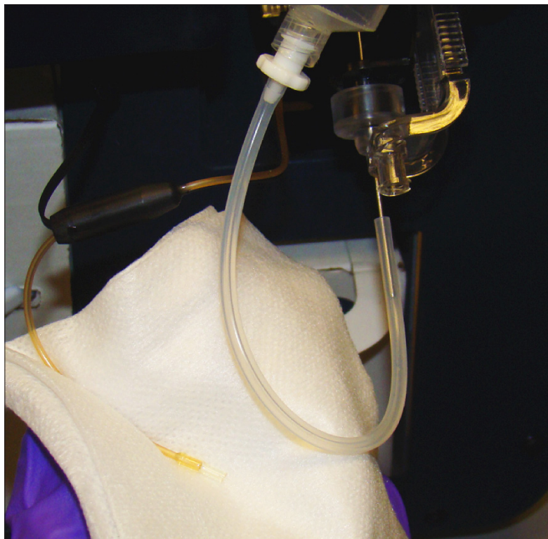
Figure 7.6 Flushing the S-Line
