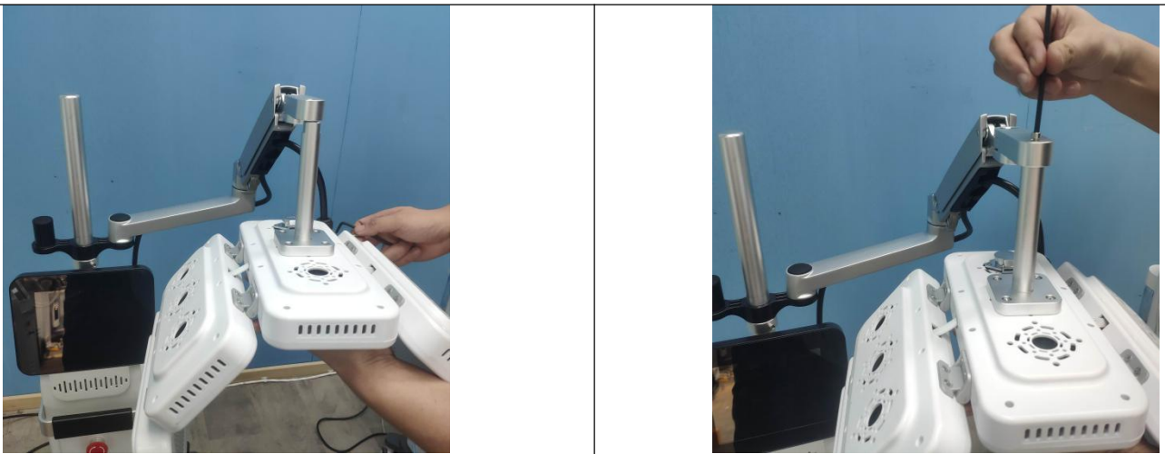
Step14: Install the light on the machine and then fix them with screws.
