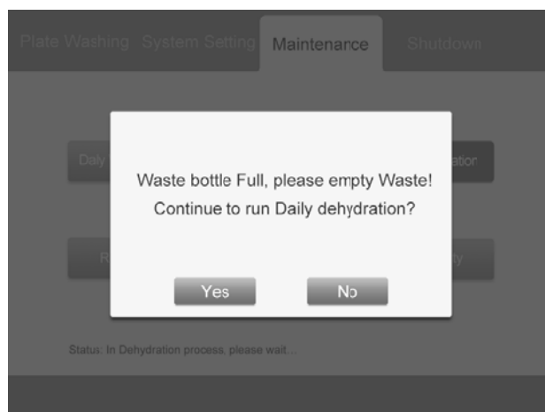
3-19 Alarm of Full Waste Liquid Container in Dewatering
